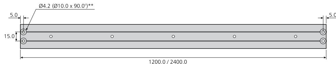
\* Fixing: drill 4.2mm holes on centre line, fully countersunk.
